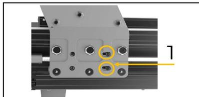
After long term use, the screw travel of the spindle may be abnormal. So you have to remove the side cover of the machine, loosen both fixing screws (1) (→ the spring returns to its original position) and then tighten the screws again and remount the side cover.
