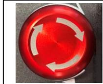
A self-locking Emergency Stop button to stop dangerous movements at any time.
